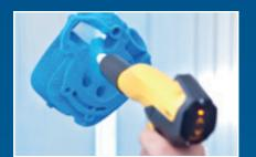
On-gun remote control gives the flexibility to adjust parameters without turning away from the work.
